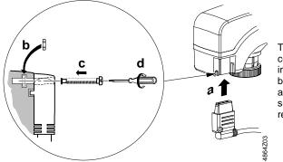
The cable connector snaps into position, but can be additionally secured with the retaining screw.
